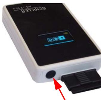
The unit is controlled by the button on the top of the unit. The button has two functions depending on how long it is pressed:
