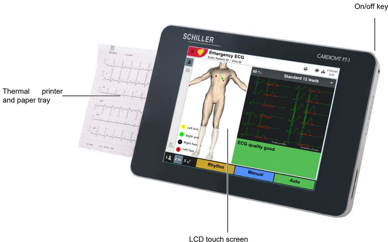
The **FT-1 Streamer** communicates with the program via a USB cable connected directly to the PC. When attached to the CS-104, the FT-1 acts as an ECG amplifier and all recording functions are carried out by the CS-104. The message **'Ready for streaming'** is displayed on the screen. This changes to 'Streaming' when transmitting data.
