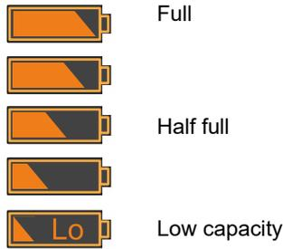
The battery symbol in the lower left of the screen indicates the battery status. When the battery is full the symbol is filled.
