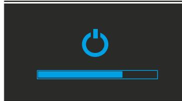
At the end of the time-out period, the off icon is displayed flashing in the middle of the screen for a few moments and the unit is switched off.
