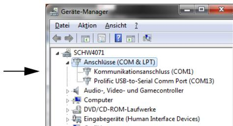
Connect the RS-232 Serial Adapter. After a few seconds four extra ports are displayed. These are the four ports of the adapter.
