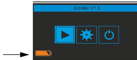
When the low capacity icon is displayed, battery capacity is limited and the batteries should be changed. Because of the high energy efficiency of the unit however, there may still be several hours of use after the low battery indicator is given.
