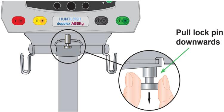
3. Release the lock pin and ensure it locates in the hole in the mounting plate. This can be verified by attempting to slide the Ability unit sideways. ***It must be securely locked into position.***
