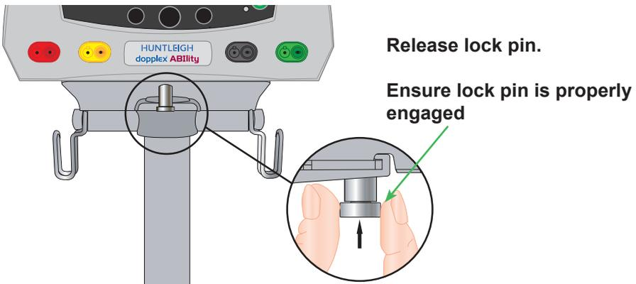
**CAUTION:** Ensure that the Ability unit is securely fitted to the roll stand and that the lock pin is properly engaged.
