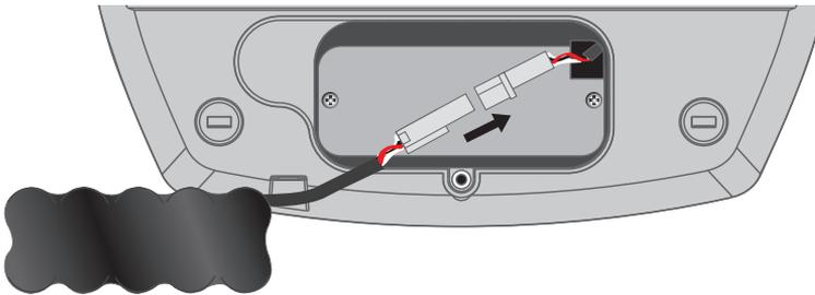
3. Replace the battery. Re-fit the battery cover and replace the securing screw with the allen key provided. **DO NOT OVERTIGHTEN!**
