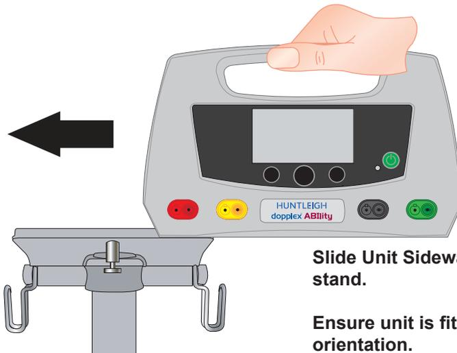
**Slide Unit Sideways onto the roll stand.**
