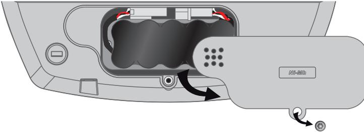
2. Lift the battery out, and connect the battery to the unit.
