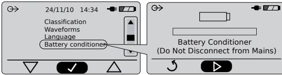
If Battery Conditioner is selected when mains (line) power is not connected, the following message is displayed:-
