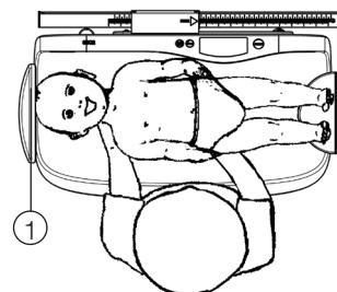
1. Lay the baby on the weighing tray. The baby's head must be at the head stop (1) of the tray.
