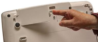
5. Remove the battery from the compartment.
